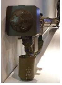
FN-6 with close up on Thermal Battery
